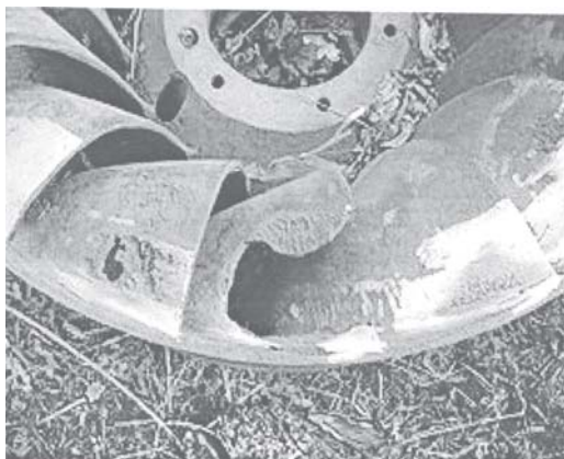
Fig.1. Cavitation damage to a Francis turbine
