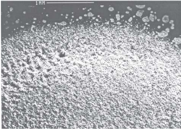
Fig. 4. General view of the cavitated area
